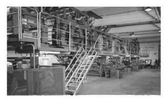
Figure 1. Conventional gravure press for laminate flooring.
